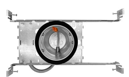
The EnVision LED 4" can is suitable for use with EnVision LED 4" models that are available in various selections. Choose the correct can for your application with our remodel or new construction version. Both cans are IC-rated and have an LED quick connect input.
