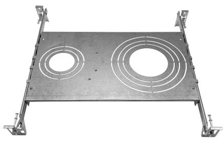
The Envision LED universal mounting plate, fits 1", 2", 3", 3.5" 4", 5" and 6" recessed light kits and is the perfect choice for new construction and remodeling. Each mounting plate come with 2 hanger bars which can extend from 13.5" to 25.5" and a plate that can slide along the bars from end to end. Made of durable metal so you can be sure your recessed lighting is secure.
