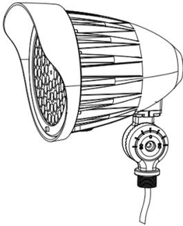
2. Thread the fixture into the cover plate (not provided), screw the hex nut (provided in the accessory bag), and face the fixture in the preferred direction.
