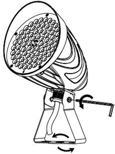
3. Install the fixture on the ground or mounting plate (not provided) through the mounting holes on the bracket (2.36"-3.14" distance between the two mounting holes).
