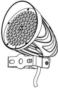
2. Loosen the bracket screws to make it adjustable.
