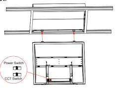
5.As shown in the figure, the retrofit kit troffer body is suspended and hooked to side-mounting bracket, make sure it is clampled tightly.
