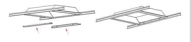
4. Hook the retrofit kit troffer body to the existing frame through the clasps in body to the side-mounting bracket.
