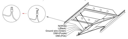
8. Rotate the retrofit kit troffer body upward, push it to the surface of side-mounting bracket.
