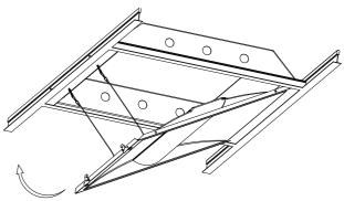
9. Push the retrofit kit troffer body to secure latches, until hearing a "click" sound to ensure it fastened tightly.
