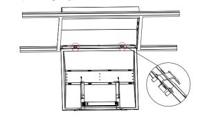
6. Hook the retofit kit torffer safety rope to the hole of corresponding side-mounting bracket, suspend the retrofit kit troffer body
