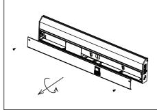
Insert the plastic expansion pipe from the accessory package into the installation plate.
