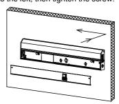
Take out the plastic expansion pipe from the accessory package and insert it into the installation plate.
