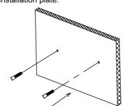
Insert the mounting hole of the lamp into the screw head and move the lamp to the left, then tighten the screw.
