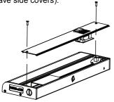
4. Insert the wire into the lamp body and then use a Phillips screwdriver to install the upper cover.
