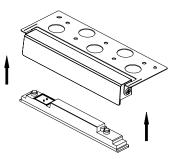
Take the right direction, put the new light module into groove (magnetically mounted )
