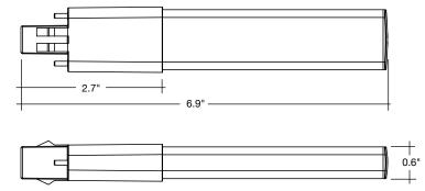
EnVision LED has manufactured a 2-PIN GX23 PL lamp replacement in LED that can work with or without the existing ballast. With a 360° angle, replace existing fluorescent G24 lamps in either vertical or horizontal direction. Unlike fluorescents, our LED lamp does not need time to warm up, it turns on instantly.
