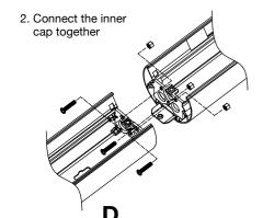
Step 1. Use the screw 3xUNC8-32 connect the inner end
