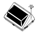
11.Fix the fixture with screws.
