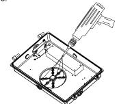
5. Drill through the mounting hole with an electric drill.
