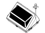
2.Use a screwdriver to remove the screws on both sides.
