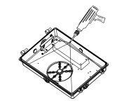
4.Drill through the mounting hole with an electric drill.
