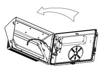
3.Open the fixture, disconnect the connection terminals, and remove the upper cover of the fixture.
