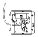
9. The top terminal connect the wire tube through the side hole to the L,N and G wires on the power supply.
