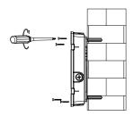
8.Push the expansion rubber plug into the mounting hole on the wall
