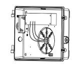
7. Thread the wire through the bottom hole.
