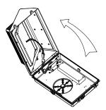
3.Open the fixture, disconnect the connection terminals, and remove the upper cover of the fixture.
