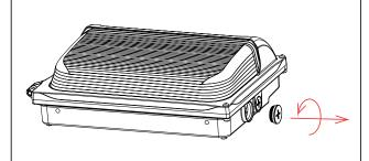
5. Unscrew the cover of the entry hole on the lamp base and remove the cover.
