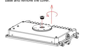
Put the input line in the embedded box passes through the waterproof pad and then passed through the lamp base.
