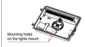
8. Use screw to lock the lamp base on the embedded junction box and ensure the balance of the horizontal column.
