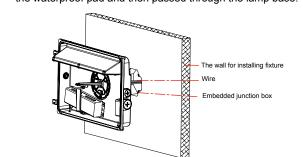
Connect the input wire and the dimming wire of the light, then put the connected wires into the embedded terminal hox
