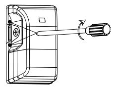
8. Make sure wiring and screws are placed tightly, then turn on power.
