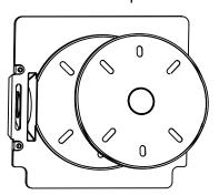
4. Screw the bottom plate on the wall
