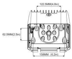
Make mounting holes on the wall according to the size shown in the picture. Use an electric drill to drill through the mounting holes on the lamo.
