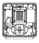
8. Connect the wires correctly and protected correctly. Pull out the wire connected to photocell if photocell function is not demanded.
