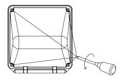
2. Unscrew the 4 screws of the lamp cover and the rubber sleeve on the screw must be discarded
