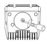
4. Remove the 1/2" plug with a screwdriver
