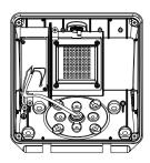
Connect the wires correctly, make sure wires are protected. Pull out the wire connected to photocell if photocell function is not demanded.
