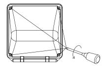
Unscrew the 4 screws of the lamp cover and the rubber sleeve on the screw must not be disacrded.
