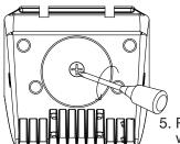
5. Remove the 1/2" plug with a screwdriver
