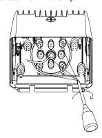
7. Drill the mounting holes of the mounting plate with an electric drill and screw the lamp onto the mounting plate.
