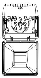
3. Remove the lamp cover, careful not to damage the lamp cover.
