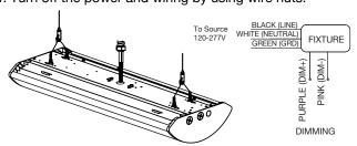
5. Insert the conduit and conduit fitting into the lamp housing. Please find the suitable conduit and conduit fitting for branch circuit connection.
