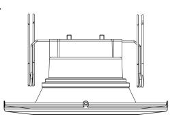
3. Flatten each protruding part that fixed on the downlight.
