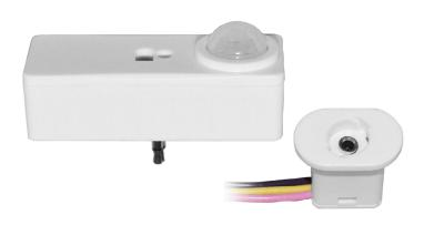
S-AUD-PIR-SL allows for individual luminaire control and is equipped with both occupancy + daylight sensing. It utilizes a Bluetooth® Low Energy (BLE) mesh network. Commissioning can be set through the SILVAIR mobile app or desktop site.
