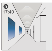
The light automatically turns on at 10% when natural light is insufficient (no motion)
