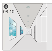
When the natural light level exceeds set point off to light, the light will turn off even when the space is occupied.
