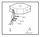
Turn OFF/disconnect power at circuit breaker. Typical junction box wiring has only white and black switched wires controlled by wall switch for ON/OFF or dimming. Ensure the junction box has an additional set of unswitched wires (continuous) main power wires as shown.
